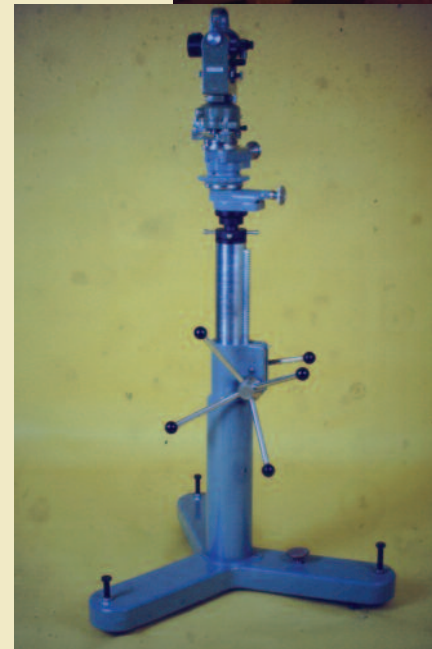
Above: the Wild T2 was just as at home on the shop floor as it was on the construction site or mapping in the wilderness. The image shows an engineer using the T2 with the GAP1 prism for auto collimation. The image on the left shows a high precision industrial stand with the theodolite on top.
