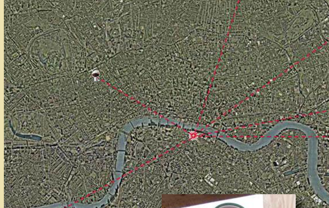
Above: local stations within the Leica SmartNet system enable the GNSS receivers on the slipform rig to provide the best possible positional data for the engineers.
