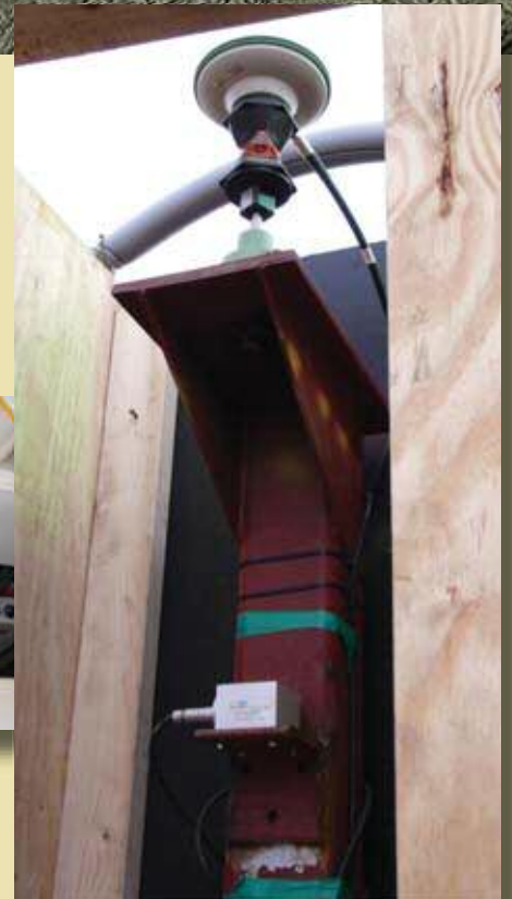
Above: four GMX902GG GNSS Receivers inside the continuously moving slip form rig building the central core of the Shard. Right: Co-located with the GNSS receivers is a Leica AS10 GNSS Antenna, 360^\circ prism and dual-axis inclinometer.
