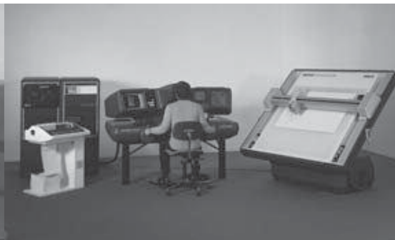
Wild was using computers to solve surveying and photogrammetry problems from the early days but the arrival of computing power in the late 1960s drove many new developments. We shall learn more about photogrammetry in the next section of this history. Below from left to right: the Wild EK8 computer introduced in 1968, a Wild A9 stereo plotter, (1957-72), Wild AC1 Analytical Stereo Plotter and TA2 Plotting Table launched in 1980, the Wild BC1 launched in 1982.
