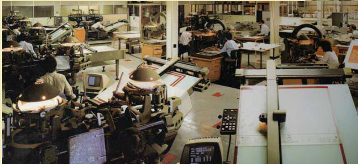
Below: Map production from stereo aerial photography. The heart of BKS Surveys before the digital age.
