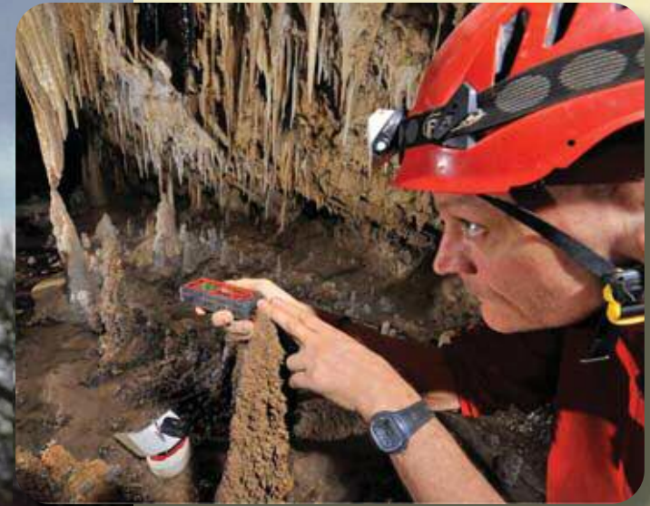
Above: a caver uses a Leica DISTO D2 to capture data for a cave survey.
