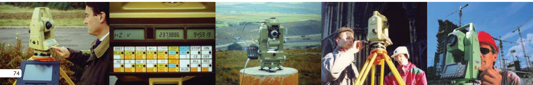
Below from left to right: Tim Badley puts a TC500 electronic total stations connected to a Grid tablet computer through its paces. The keyboard of a TC 2000. A T16, Distomat and data recorder sit atop a Triangulation Pillar. A Wild T2000 electronic theodolite connected to a Distomat and keyboard is the ideal combination for this crew capturing details for monitoring Ely Cathedral. The Leica TPS 300 launched in 1998 marked a new era for the total station..
