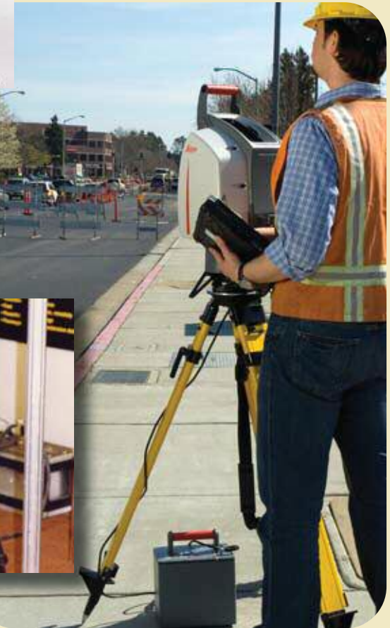
With the arrival of laser scanning an old problem for surveyors returned: external batteries. Back in the 1960s when EDM first arrived surveyors were forced to use 6 and 12 volt car batteries for their power source. The early laser scanners were similarly power hungry until Leica Geosystems got on the case and developed smaller batteries and clever power management.
