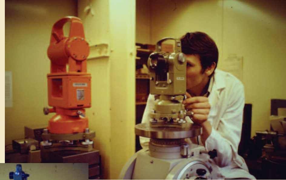
Above: the Wild T2 was just as at home on the shop floor as it was on the construction site or mapping in the wilderness. The image shows an engineer using the T2 with the GAP1 prism for auto collimation. The image on the left shows a high precision industrial stand with the theodolite on top.
