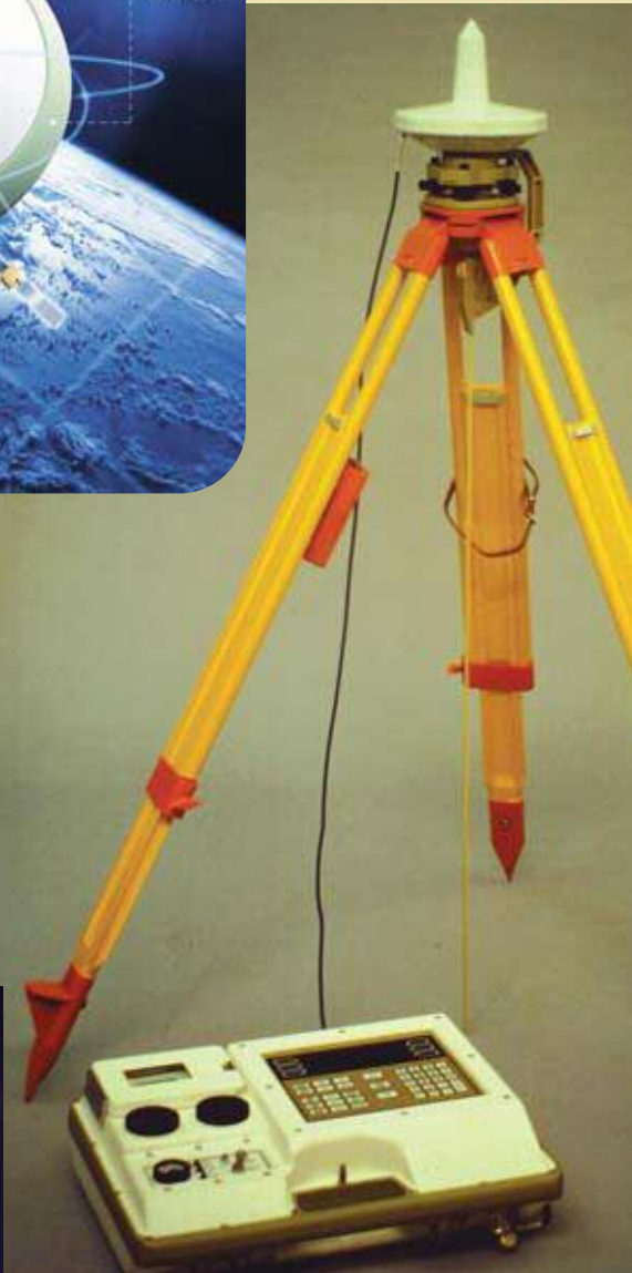
Right: no, it's not a 1980's ghetto blaster with a handy antenna for better reception but the dawn of GPS Surveying, the Wild WM101.
