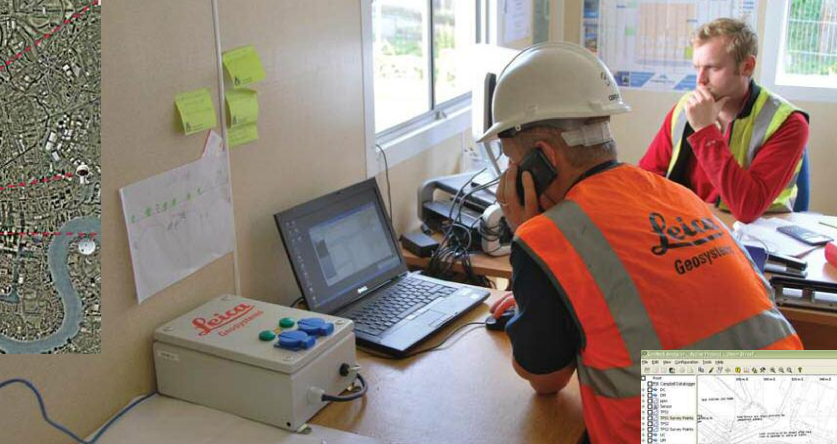
Left: At the Shard James Whitworth analyzes data received from GPS and other sensors by the Leica GeoMoS software.
