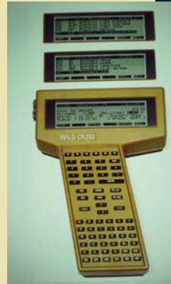
Right and above: the Wild CR299 GPS controller was the essential tool for GPS surveys.
