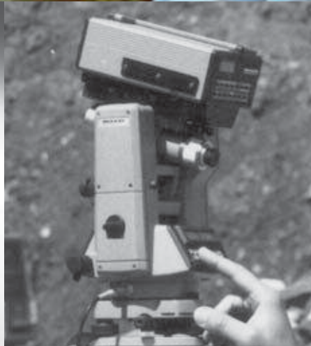
Main image, a Wild APS system comprising a TM3000V motorised electronic theodolite incorporating video, DI3000 Distomat and datalogger. Note the Joy Stick control! Bottom of page: TC1, TC1000, TC2000 total stations, DI3002 Distomat and GRM10 Rec Module for data logging with GIF10 Reader to interface with a PC.
