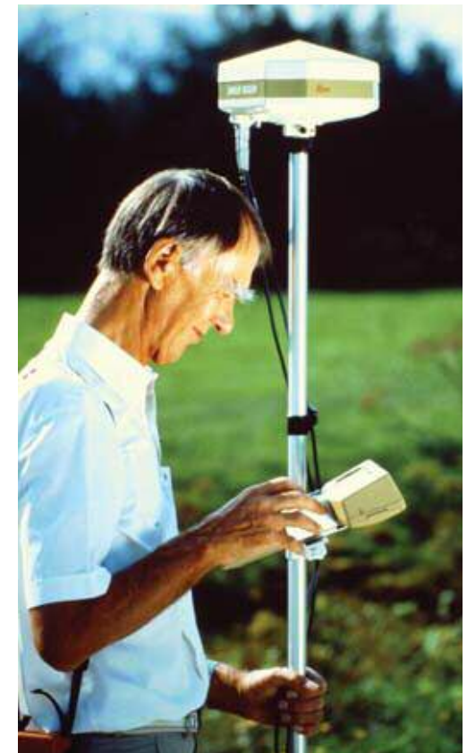
Images opposite: the first GPS constellation, while a surveyor operates an early Wild-Magnavox GPS receiver. Alas, GPS surveying was a bit like “Waiting for Godot” - it could take hours to get a fix.
