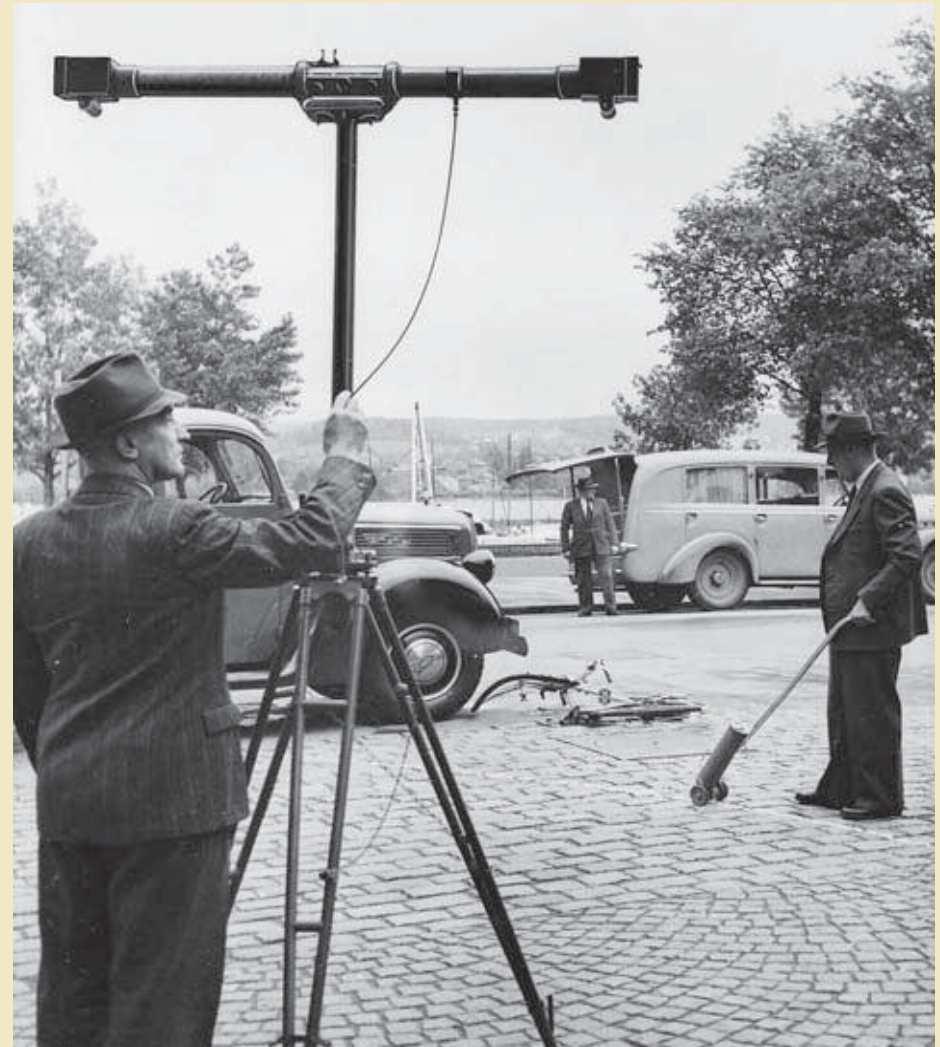
Below: even before the second world war Wild had developed a stereometric camera, here shown capturing a scene from a road traffic accident.
