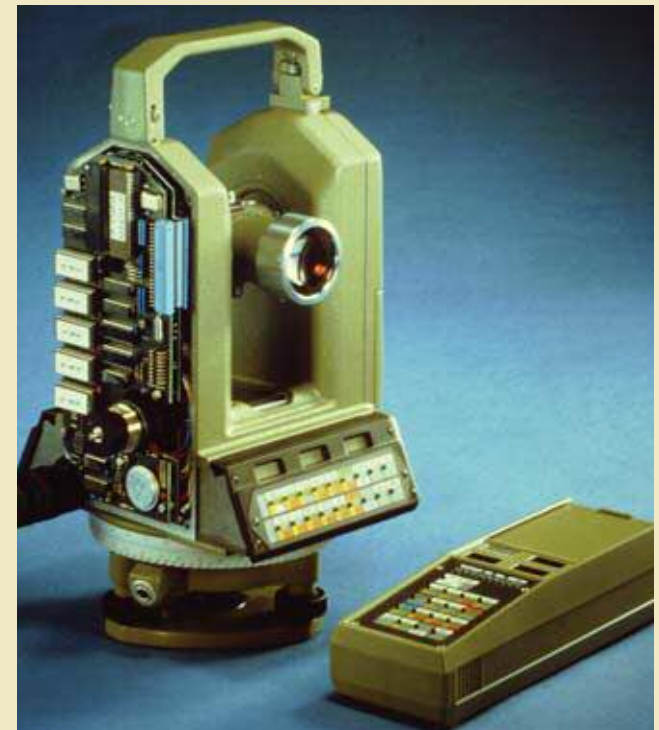
Above: at last surveyors had an all-in-one instrument. The Wild TC1 total station was launched in 1977.
