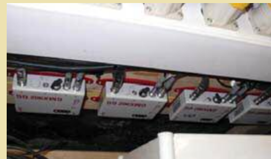
Above: four GMX902GG GNSS Receivers inside the continuously moving slip form rig building the central core of the Shard. Right: Co-located with the GNSS receivers is a Leica AS10 GNSS Antenna, 360^\circ prism and dual-axis inclinometer.
