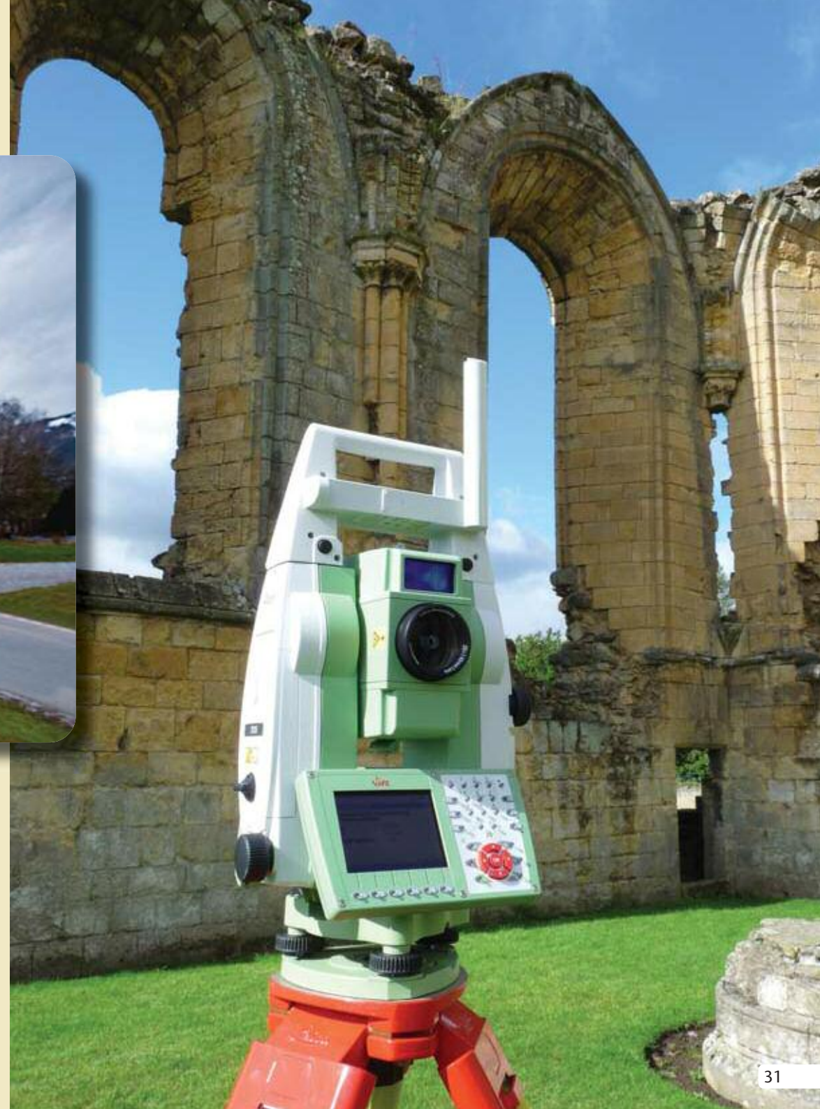
Right: the heritage sector has become major users of surveying equipment. This Leica TS15 total station is seen at Byland Abbey.
