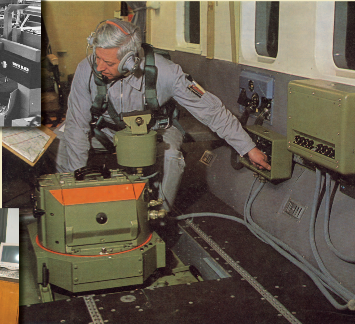
Above: the plotting room at Ordnance Survey in the 1970s. In the foreground an operator is working at a Wild A10 Autograph.
