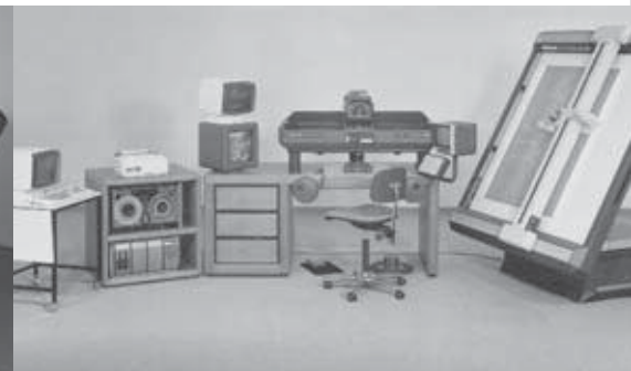
Wild was using computers to solve surveying and photogrammetry problems from the early days but the arrival of computing power in the late 1960s drove many new developments. We shall learn more about photogrammetry in the next section of this history. Below from left to right: the Wild EK8 computer introduced in 1968, a Wild A9 stereo plotter, (1957-72), Wild AC1 Analytical Stereo Plotter and TA2 Plotting Table launched in 1980, the Wild BC1 launched in 1982.
