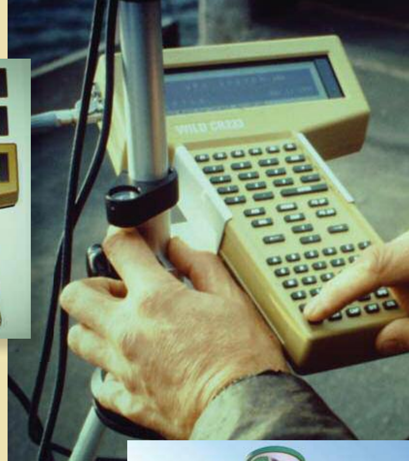
Right and above: the Wild CR299 GPS controller was the essential tool for GPS surveys.
