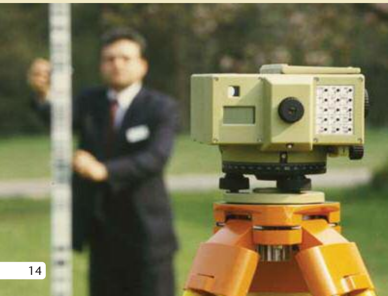
Below: a smart young staffman (Nigel Bayford) demonstrates the Wild NA2000 bar-code reading digital level.
