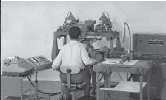
Wild was using computers to solve surveying and photogrammetry problems from the early days but the arrival of computing power in the late 1960s drove many new developments. We shall learn more about photogrammetry in the next section of this history. Below from left to right: the Wild EK8 computer introduced in 1968, a Wild A9 stereo plotter, (1957-72), Wild AC1 Analytical Stereo Plotter and TA2 Plotting Table launched in 1980, the Wild BC1 launched in 1982.
