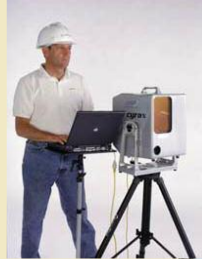
Left: the Cyrax 2400 laser scanner was a pioneering development for surveyors and engineers. In the early models however control from a laptop was essential as was an external battery.
