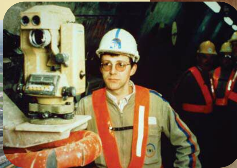
Left: a Eurotunnel surveyor checks a measurement from a permanent fixed plate with a Wild T1600 surmounted by a Distomat. Below: tunnel surveyors check the tunnel bearing with a gyro, the Gyromat 2000 incorporating a Wild T2.
