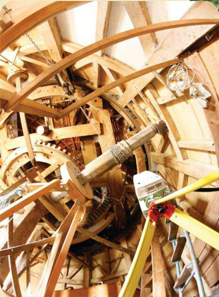
Above: this old windmill would have been a serious challenge to capture all of the detail in 3D and would have taken days of measurement. No problem now with a Leica HDS scanner.
