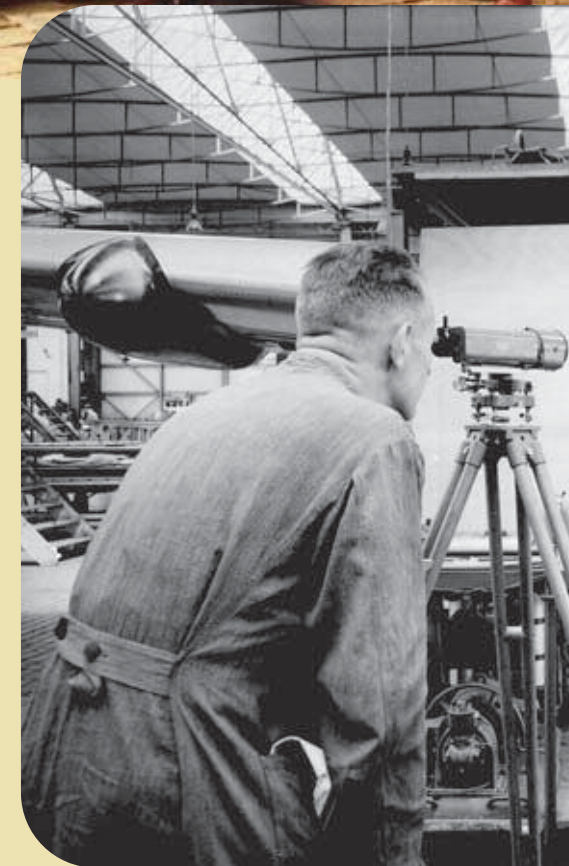
Right: Keep level and fly right - an engineering level is used to check the wings of an aircraft. According to the records, this image predates the founding of Wild UK by four years. The inset image (right) shows the same work today being done by a Leica T-Probe, similar to the one opposite above the Red Bull F1 car, for Airbus Broughton.
