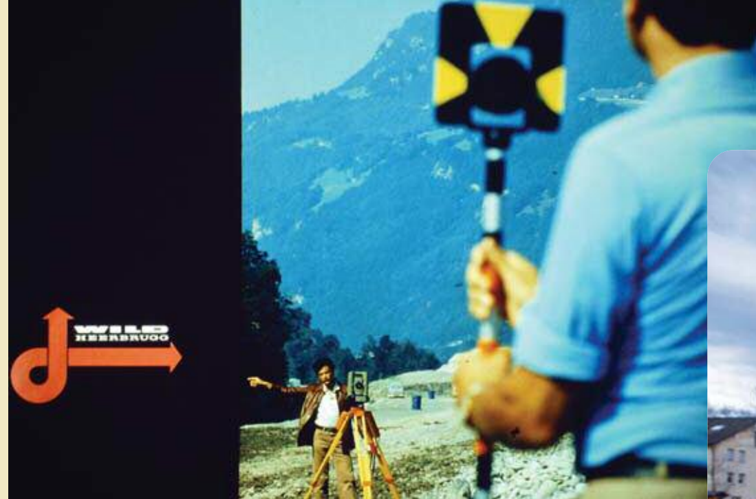
Above: at last surveyors had an all-in-one instrument. The Wild TC1 total station was launched in 1977.
