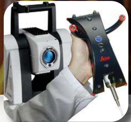
Below: Leica Geosystems now shares its new headquarters with Hexagon's Metrology division whose customers include the Formula 1 teams like Red Bull. Inset image shows the Leica Geosystems' Universal CMM, part of a coordinate measuring system.
