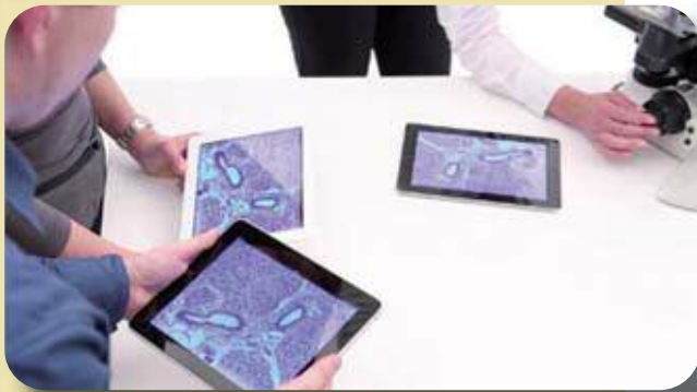
Above: Multiple iPads can be connected to the same camera so that the user can share live images.
