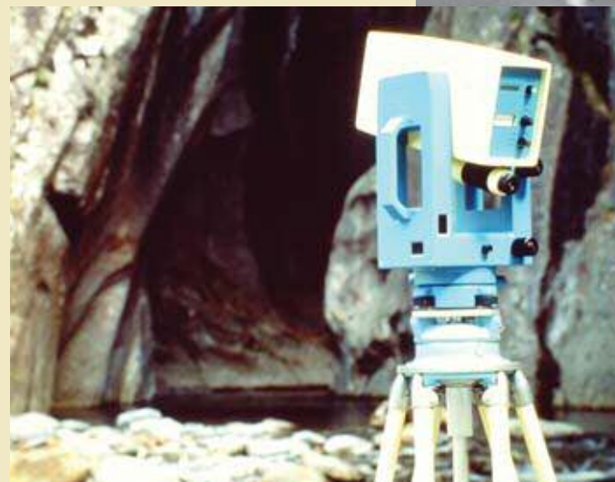
Above: an embryonic total station combines a T2 and DI10, while an inquisitive camel and puzzled boy look on. Below: the state-of-the-art Kern Mekometer EDM.
